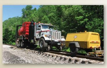
The Hulcher air evacuation service is an excellent fit for work around the hump yard, railroad signals and on the right-of-way. Air excavation cleans retarders, switches and crossings, loosening mud and fouled ballast quickly and cost effectively. It is also an excellent solution for exposing underground utilities. Air excavation works perfectly with a Hulcher hi-rail vacuum truck, which collects the loosened debris for reuse or disposal.
